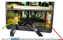
Fig. 12.1 Auxiliary Switch Assembly (inside control box)
